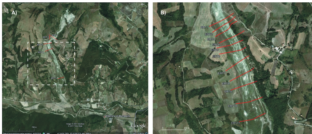
Fig. 2 – Electrical resistivity tomography surveys carried out on the Montaguto landslide on July 2011 (A) and October 2012 (B).
