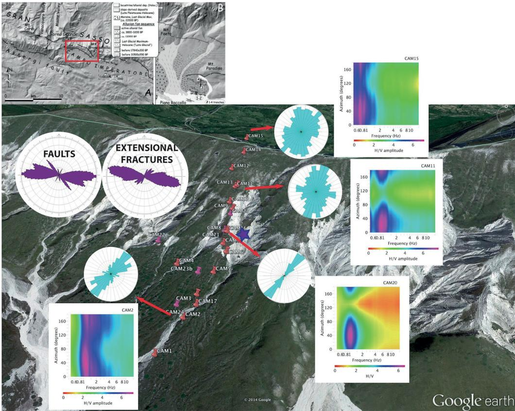
Fig. 3 – Ambient noise polarization at four stations installed across the Campo Imperatore normal fault (CAM2, CAM11, CAM15 and CAM20). At each station the rose diagram (cyan) obtained by the covariance matrix analysis are drawn as well as HVSR contour plots (the amplitude scale is different for each plot). The strike of faults and extensional fractures measured by a detailed geological survey at one location (violet star) are reported as well through violet circular histograms.
