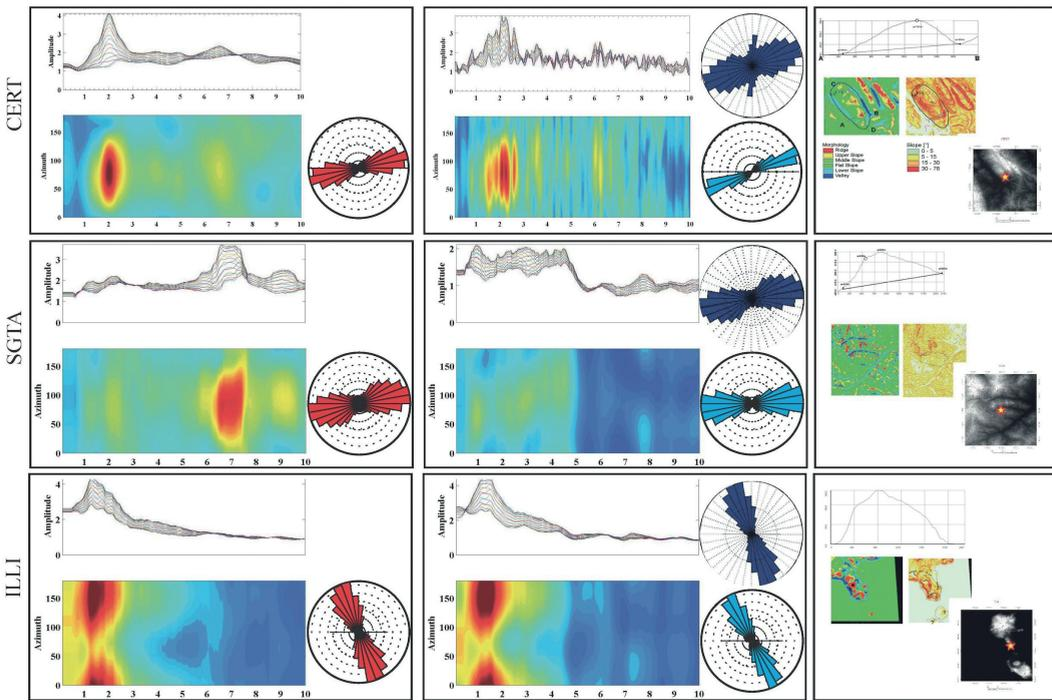
Fig. 1 – Results of polarization analysis for three representative stations. The top panel shows the polarization result at station CERT (Cerreto Laziale), on a 1 km wide and 300 m high ridge with a nearly elliptical shape. This station is an example of a systematic directional amplification occurring transversally to the topographic elongation. The middle and bottom panels represent results from stations SGTA (Sant’Agata Puglia) and ILLI (Lipari), respectively.
