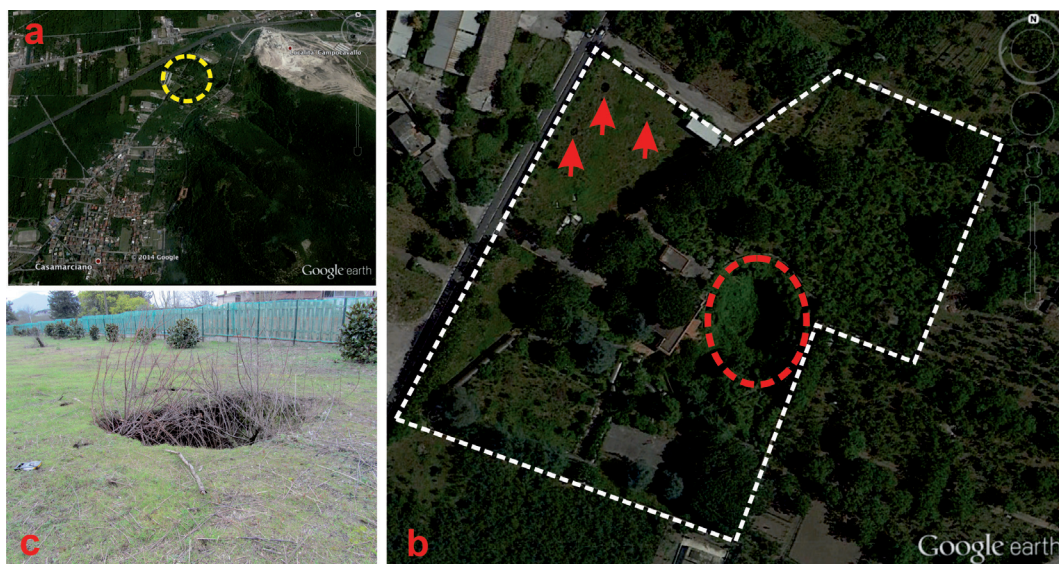
Fig. 1 – a) Aerial photography with location of the survey area by Google Earth (yellow dotted line); b) survey area on Google Earth aerial photography (white dashed line) with some surface evidences of sinkhole (red arrows) and larger sinkhole in the area (red dashed line); c) photo of some surface evidences of sink-hole.
