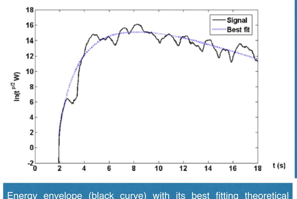
Energy envelope (black curve) with its best fitting theoretical model. Single path Qi and Qs parameters are the parameters of the best fit curve
