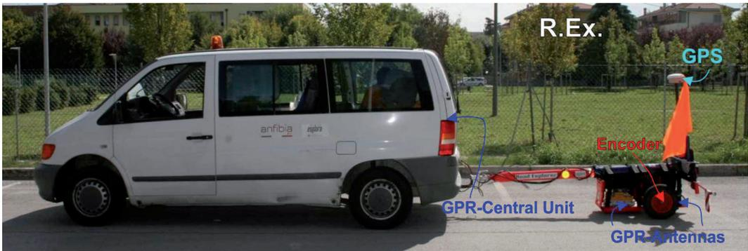
Fig. 1 – R.Ex. GPR system and its components connected to a van during a survey.
