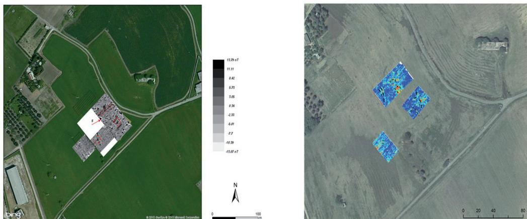
Fig. 2 – The GPR and magnetic gradiometric surveys in Cutrofiano allowed the identification of buried walls and structures of probable archaeological interest. Structures seem to have same alignment SE-NW.
