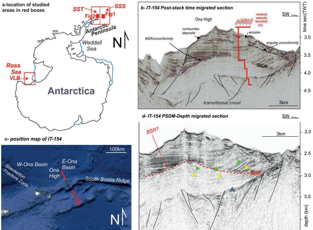
Fig. 1 – a) location of the study areas: SSS-South Scotia Sea, SST-South Schetland Trench, VLB-Victoria Land Basin; b) portion of seismic profile IT-154 crossing the Ona Basin-Ona High (location in c), where the red line represents the interval velocity trend through the observed BSR; d) pre stack depth migration where the arrows depict the continuity toward SW of sedimentary reflectors even through the BSR, while toward NE the BSR seems to coincide with an unconformity.
