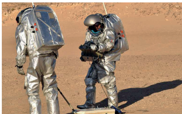
Fig. 1 - Analogue astronauts collecting GPR data during the ScanMars experiment of Amadee18 (Photo credits OeWF).
