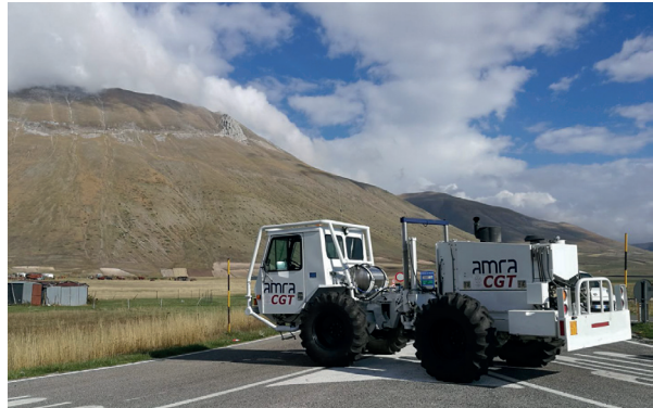
Fig. 2 - The Minivib used for the acquisition of seismic data in the Pian Grande di Castelluccio basin.
