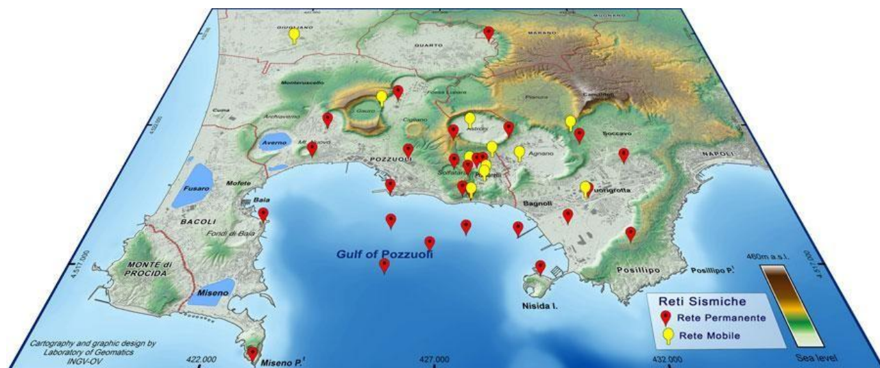
Figure 1 - The present Campi Flegrei seismic network. The map represents the permanent stations (red points) and mobile stations (yellow points). From http://www.ov.ingv.it
