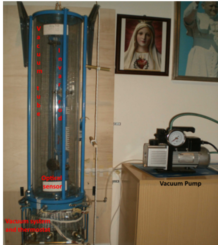
Fig. 1 – One of the damped pendulums self-built by Mario Campion in his laboratory. Note the vacuum pump connected to the base of the pendulum where the thermostat system is also located. The glass vacuum cylinder surrounds the pendulum made of invar steel. At the lower end of the rod there is a mass and the precision optical reading system of the instrument, this is connected via an optical fiber to the external rubidium clock.
