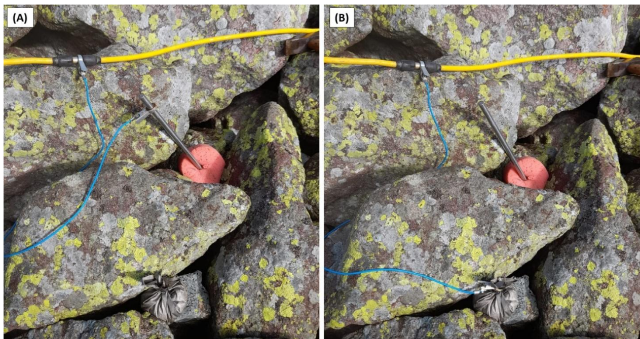
Figure 1. A) Example of measurements collected with steel-spike electrodes hammered between the boulders and coupled with sponges soaked in salt-water. B) Example of measurements collected with conductive textile sachets electrodes pushed between the boulders and wet with salt-water. Pictures realized during the comparative test performed on the inactive rock glacier of Sadole.
