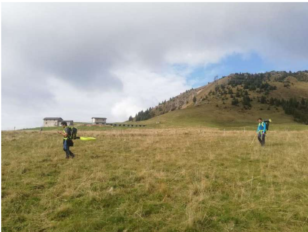
Figure 1. Loupe EM system configuration for an acquisition in the Val Sabbia (BS) mountainous area.
