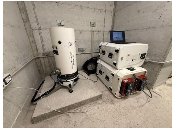
Fig. 3b – Napoli station (CeSMA). AQG-B06 gravimeter. On the left the sensor head and on the right the control units.
