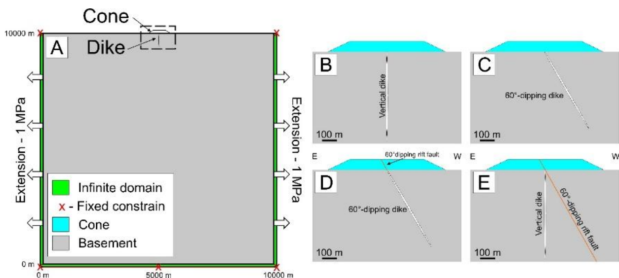
Figure 2. A) Numerical models setup; B) vertical dyke; C) 60°-dipping dyke D) 60°-dipping dyke intruding a 60°-dipping border fault affecting the cone; and (E) vertical dyke interacting with a 60°-dipping border fault.
