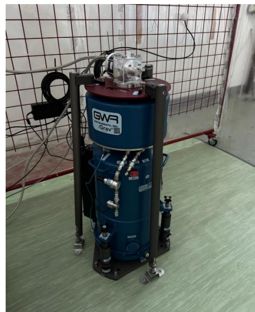
Fig. 2b – Sos Enattos station (NU). iGrav#70 superconducting gravimeter during a test in the Rimisa facility at the Sos Enattos Mine.
