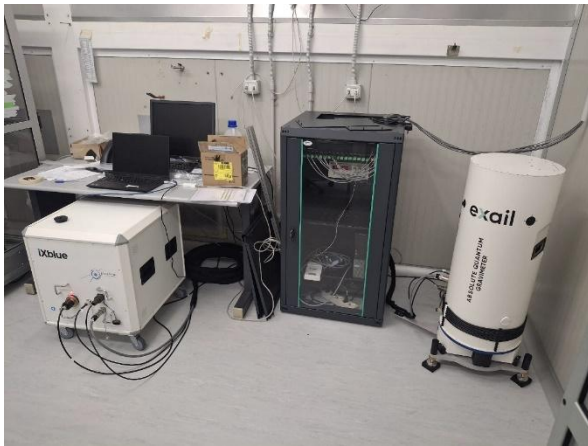
Fig. 3a – Cascina station (PI). AQG-A09 gravimeter in the clean room. On the left is the control unit and on the right is the sensor head.
