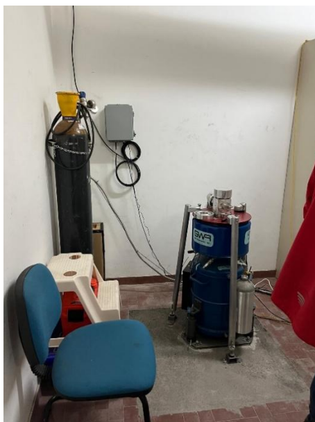
Fig. 2a – Nicolosi station (NIC). iGrav#25 superconducting gravimeter operational since 2016.
