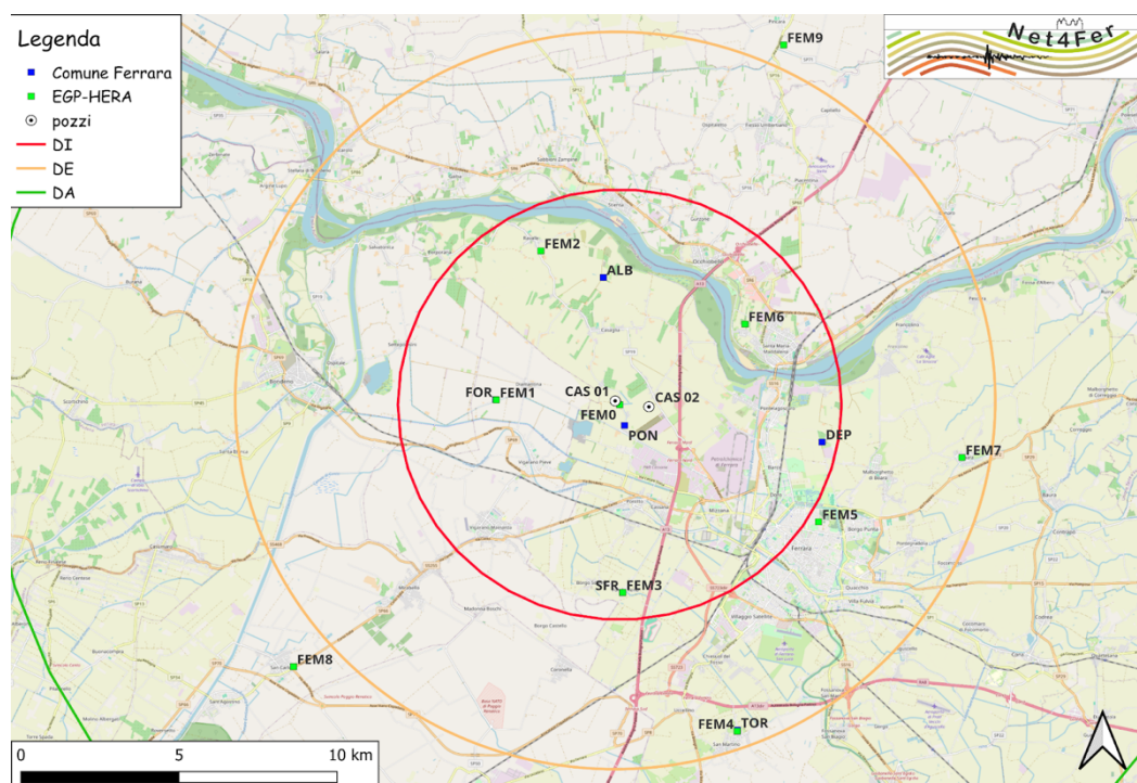
Fig. 1 – Current location of the microseismic network stations of the Net4Fer network in the alluvial plain. The stations in blue are those managed by the Municipality of Ferrara since 1990, while the more recent ones are in green ( https://net4fer.unife.it/index.php/it/monitoraggio/monitoraggio-sismico ).
