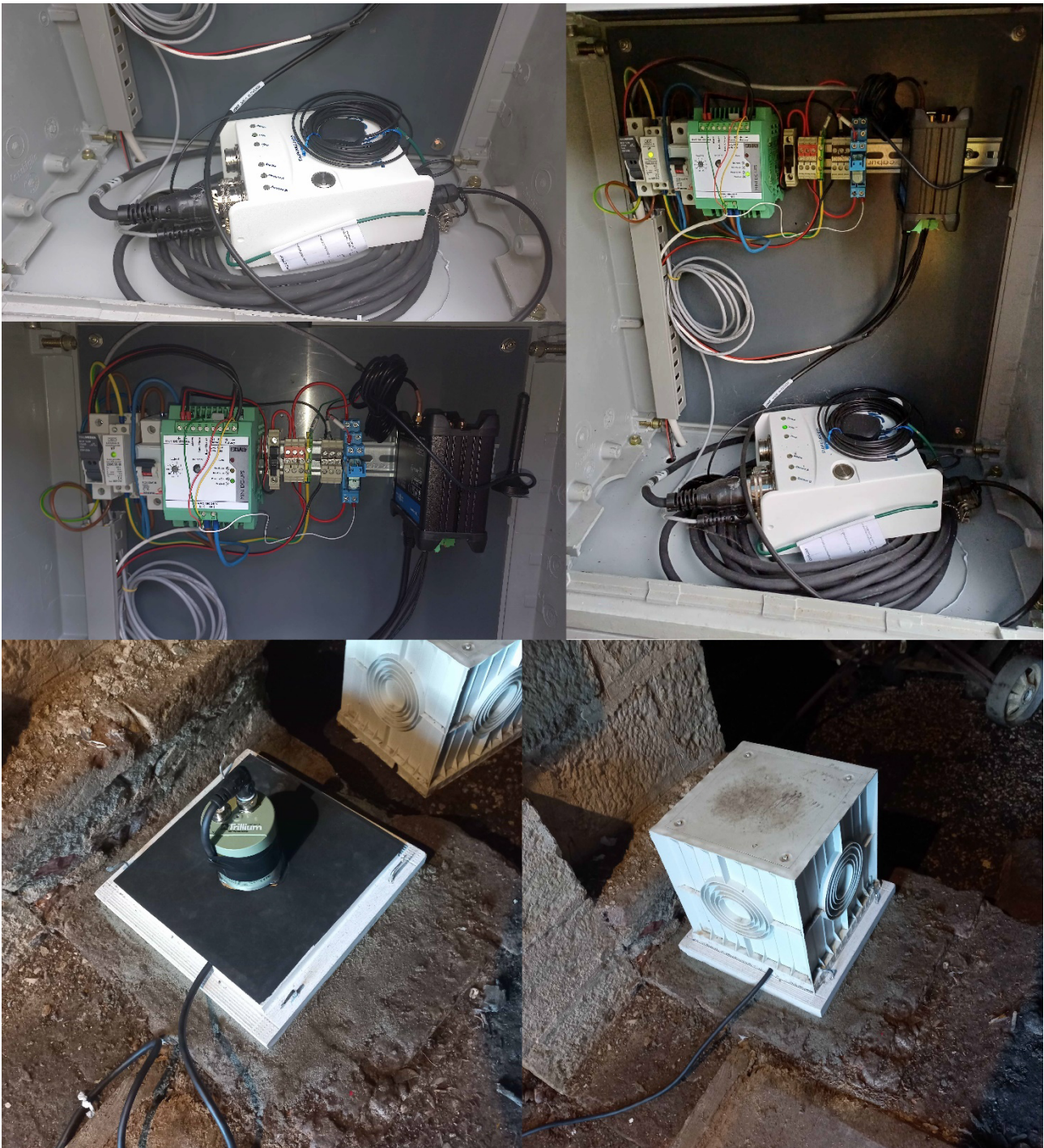
Fig. 2 – Components of an OGS seismic station for the AdriaArray project: (top left) the Nanometrics Centaur acquisition system; (centre left) the mobile internet router with switches; (top right) both integrated in a closed metal cabinet; (bottom left) the Nanometrics Trillium Compact 120 sec broadband seismometer, installed on a marble plate; (bottom right) the sensor covered with plastic thermal insulation.
