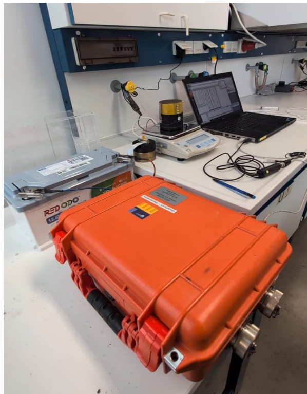
Fig. 3 – The Lab setup, composed by GeoTom resistivity meter and a Hyprop 2 (Meter group) using a customized sample holder.
